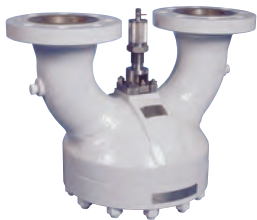
Starvalve Changeover Valves Low pressure drop COV Standard COV Combined valve with linkage system Sizes : ½" - 10" Pressure : up to 100 barg Temp : -196°C up to +427°C Mat : CS - SS
