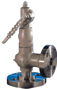
9 Series ASME Section VIII Div. 1 Portable PRV - Full nozzle Screwed/Flanged/Welded Size : ½" to 1 ½" Rating : 150# to 2500# Temp : -196°C up to +400°C
