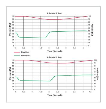
This provides the user with a high level of diagnostic data on all critical components within the actuator including the solenoid valves.
