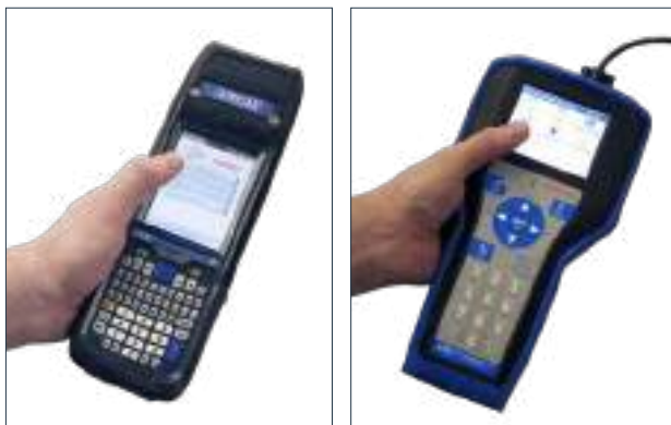
Figure 1. Left: ECOM, Right: Rosemount 475. The CVA can be configured using a Bluetooth wireless enabled device such as a PC or alternatively a typical shop HART communicator such as an ECOM or Rosemount 475
